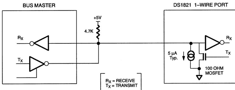
The idle state for the 1-Wire bus is high. If for any reason a transaction needs to be suspended, the bus MUST be left in the idle state if the transaction is to resume. Infinite recovery time can occur between bits so long as the 1-Wire bus is in the inactive (high) state during the recovery period. If this does not occur and the bus is left low for more than 480  $\mu$ s, all components on the bus will be reset.
